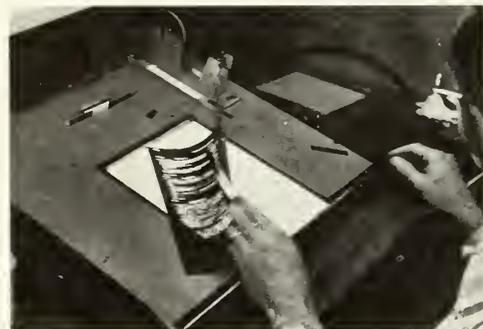
The computers transmit signals to a photocomposer, a machine that produces a negative image of a page of type, such as the one being proofed here, or a positive image.
