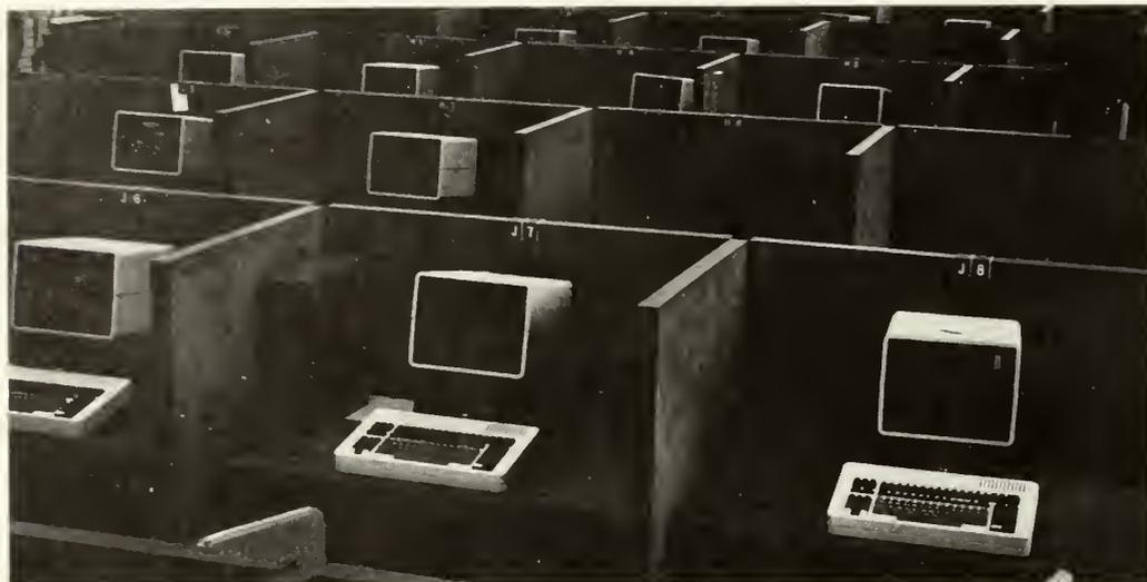
Each of GPO's computers is capable of handling output from up to 20 video terminals such as these. The terminals—75 in all—are connected by cable with the computers in a separate room.
