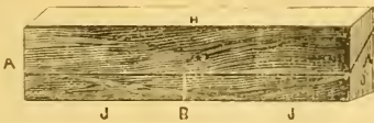
Fig. 3.—Showing how to cut sliding entrance from one piece of stuff without having to fit.
