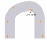
Decreasing-radius turns start out with a gentler curve, then get progressively tighter. As a result, you'll come into the corner at higher speeds than when you exit.
