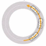
In contrast to oversteer and understeer, a car is said to be neutral if it's perfectly balanced, neither understeering nor oversteering. It is impossible for any car to be absolutely neutral in all conditions. Depending on road conditions, drivetrain layout, and horsepower, the car will exhibit different characteristics in different situations.
