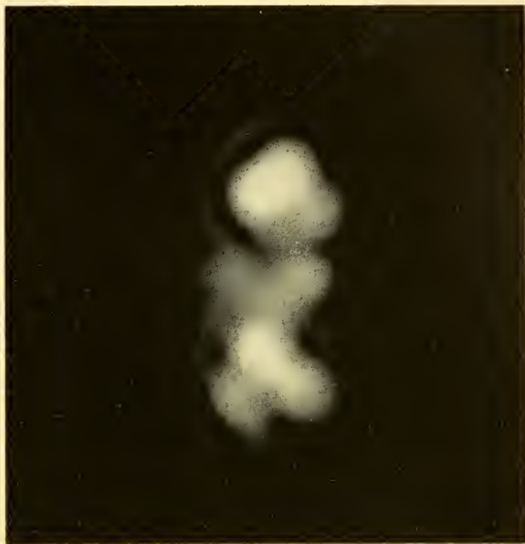
FIG. 1.66. Image structure according to the objective's N.A. n \sin u = 0.20 .
