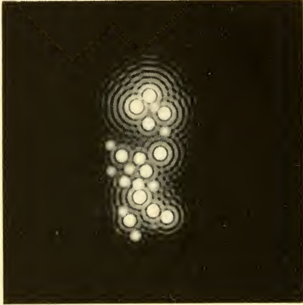
FIG. 1.68. Image structure according to the objective's N.A. nsin u = 1.30 .
