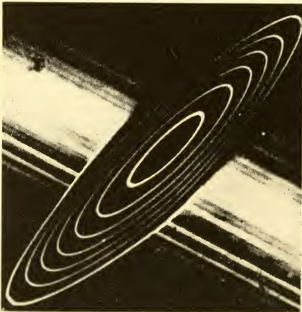
FIG. 4.37. Fringes when a small steel diamond-chip wheel is applied against a surface at a given pressure (courtesy of Prof. Tolansky).
