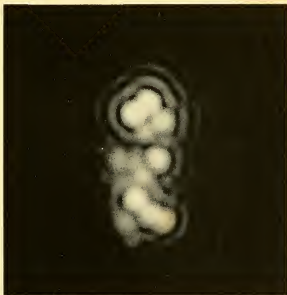
FIG. 1.67. Image structure according to the objective's N.A. n \sin u = 0.60 .
