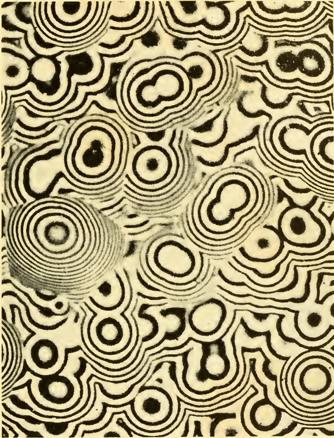
FIG. 4.25. Frosted and silvered glass surface photographed by the Zeiss interference microscope (Von Martin Uhlig. Courtesy of Zeiss).
