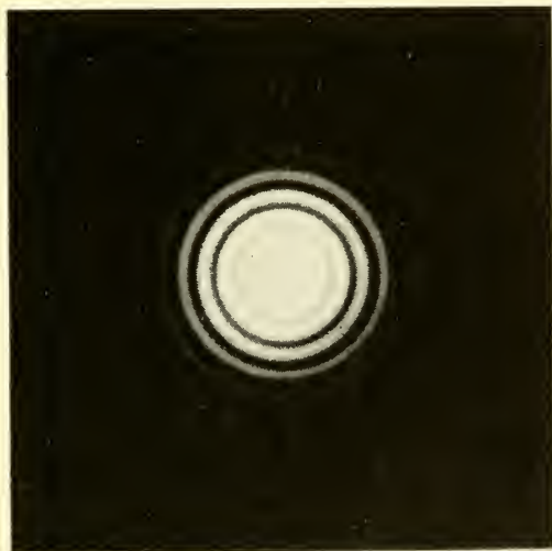
FIG. 1.11. Diffraction pattern when defective focusing has a value smaller than \lambda .
